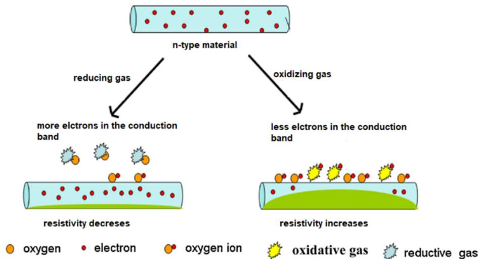
Figure 2.3: Effect of chemo-sorption of oxidizing and reducing gases on the n-type semiconductor material
