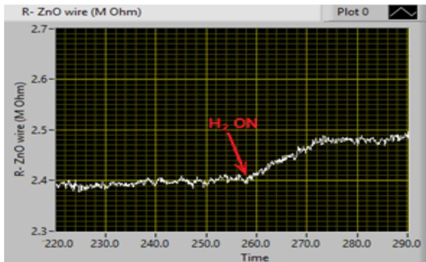
Figure 4.11: Time variation of the resistance of an individual ZnO:Sb micro-wire at 100°C due to hydrogen gas flow.
