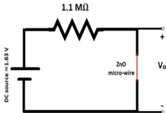
Figure 3.3 A cartoon of the potential divider circuit for the electrical resistance measurement of individual ZnO:Sb micro-wires.
