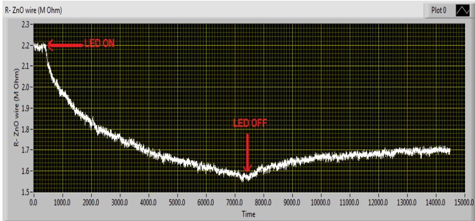
Figure 4.2: The effect of green LED, The LED was turned on at 400 sec and off at 7400 sec
