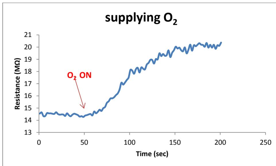
Figure 4.7: Time variation of the resistance of an individual ZnO:Sb micro-wire at 20°C due to oxygen gas flow.
