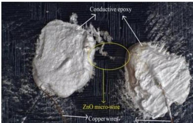
Figure 3.2 An individual ZnO:Sb : two copper wires connected to the ZnO:Sb on a glass substrate using conductive epoxy.
