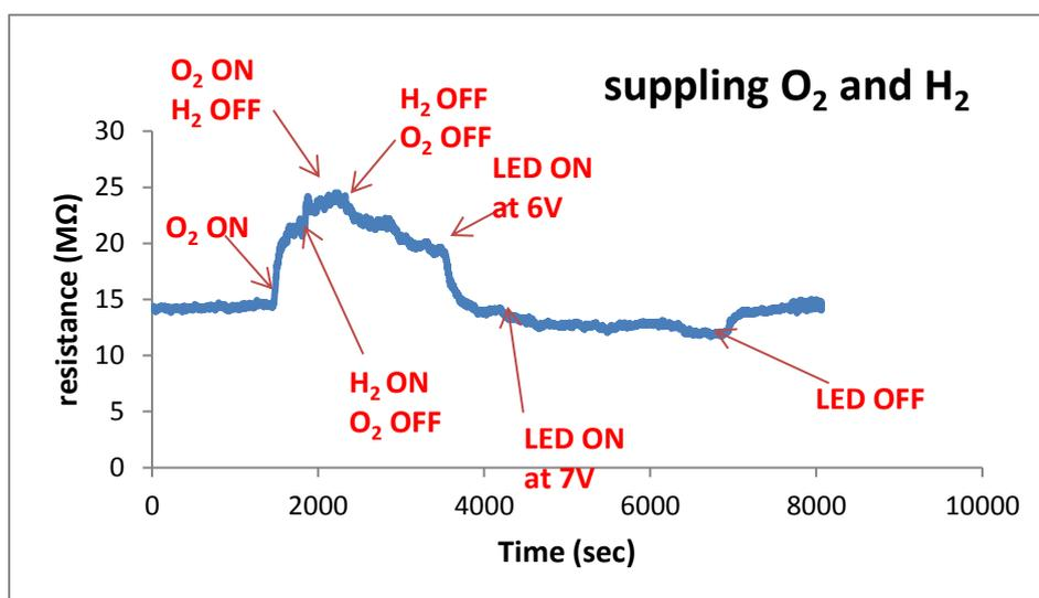
Figure 4.12: Time variation of the resistance of an individual ZnO:Sb micro-wire at 20°C due to switching between oxygen and hydrogen gas flow
