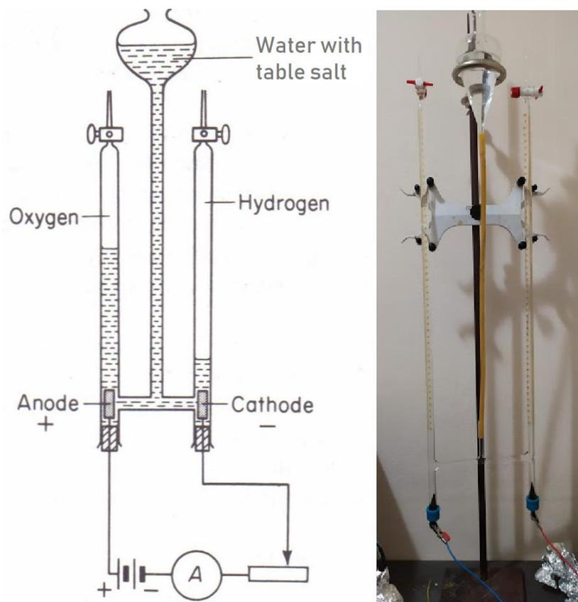
Figure 3.8: Hofmann design for electrolysis: Hydrogen gas gathers at the cathode and Oxygen gas gathers at the anode. This is the glass design.
