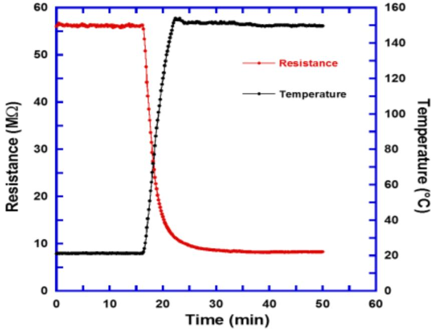
Figure 2.2: Resistance variation of a single ZnO:Sb micro-wire as the temperature rose from 20 oC to 150 oC in the absence of light[42].
