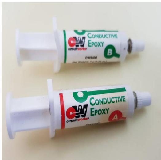
Figure 3.1 Silver conductive adhesive epoxy: A 2 part electrically conductive silver epoxy for general purpose prototype, repair and rework applications. That is quick to set, and has excellent electrical conductivity.
