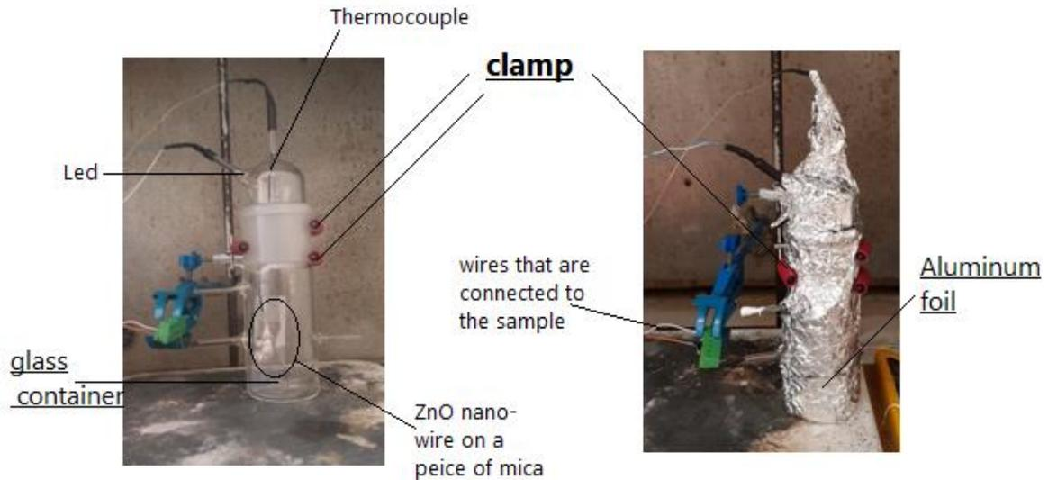
Figure 3.6: During the experiment: Left: ZnO micro-wire inside a glass container. Right: the glass container covered with aluminum foil.
