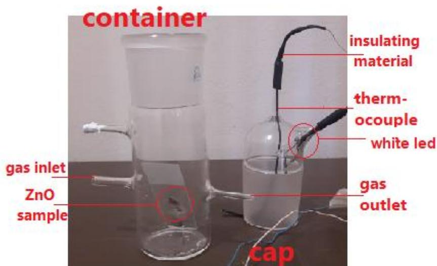
Figure 3.5: the glass container and its cap next to it: We have the ZnO sample inside the container and a hole designed to get gas inside the container, a gas outlet thermocouple and a LED.
