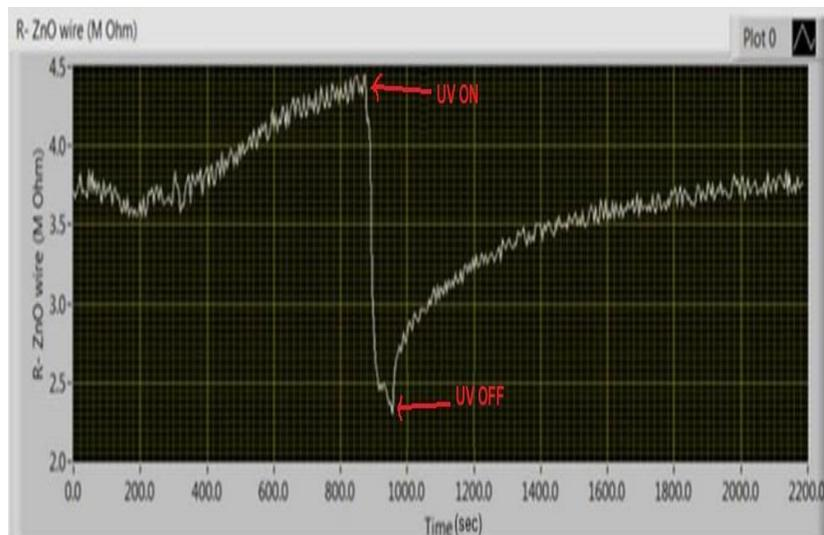
Figure 4.4: The effect of UV, The UV lamp was turned on at 860 sec and off at 960 sec.
