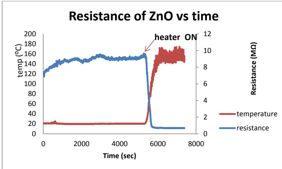
Figure 4.5: Resistance variation of a single ZnO:Sb microwire as the temperature rose from 20°C to 150°C in the absence of light. The sample was kept inside the small glass container with the cap of the container being closed.
