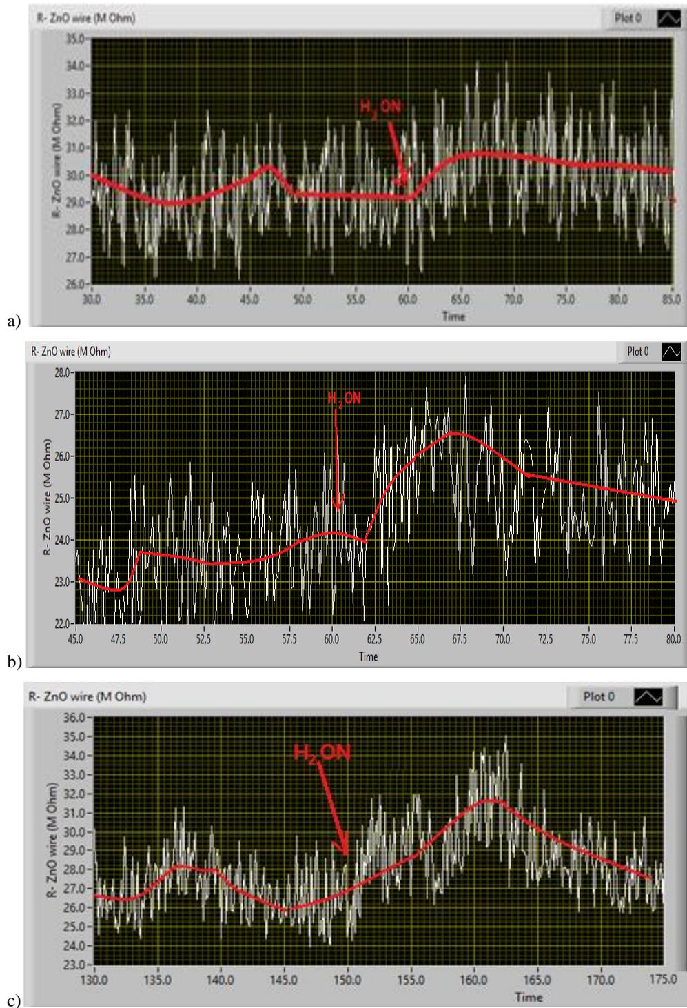
Figure 4.10: Time variation of the resistance of an individual ZnO:Sb micro-wire at 20°C due to hydrogen gas flow
