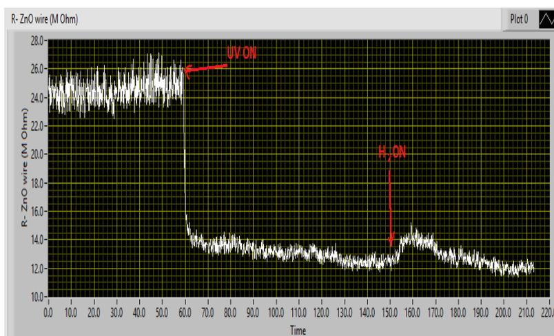
Figure 4.14: Time variation of the resistance of an individual ZnO:Sb micro-wire at 20°C due to hydrogen gas flow under UV illumination.
