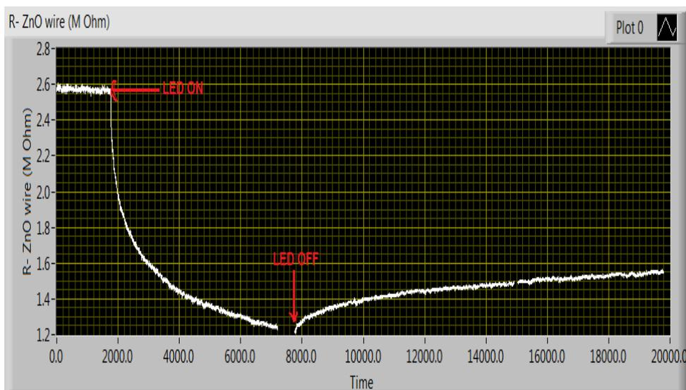
Figure 4.1: The effect of blue LED, The LED was turned on at 1990 sec and off at 8000 sec
