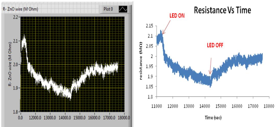
Figure 4.3: The effect of red LED, The LED was turned on at 11000 sec and off at 14400 sec, Left: the result from LabView, Right; the result drawn with excel.
