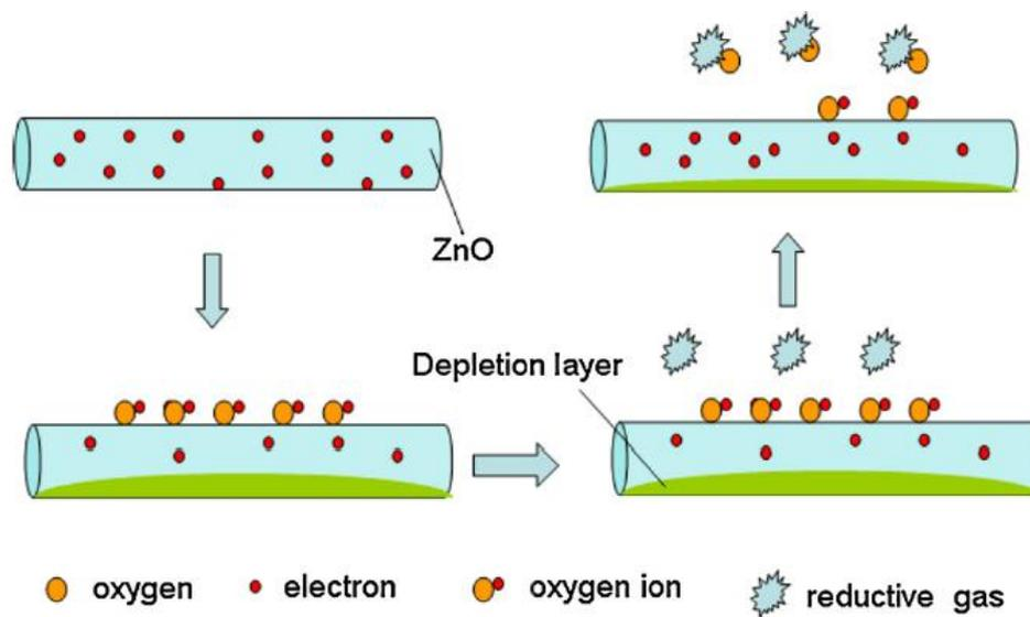
Figure 2.4: The schematic image of the reductive gas ZnO sensor [13].
