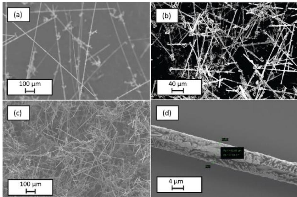
Figure 1.1 SEM images of the as grown ZnO:Sb wires: (a) about 2 cm long wires and a diameter of 5-8 micrometer, (b) about 5mm long wires and diameter of 3-5 micrometer, (c) about 2 mm long wires and a diameter of 0.1-1 micrometer, and (d) high-magnification SEM image for individual wire[24].
