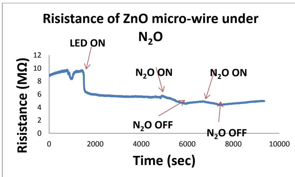
Figure 4.8: Time variation of the resistance of an individual ZnO:Sb micro-wire at 200°C due to nitrous gas flow.
