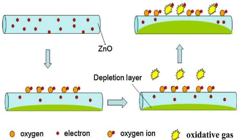
Figure 2.5: The schematic image of the oxidative gas ZnO sensor [13].
