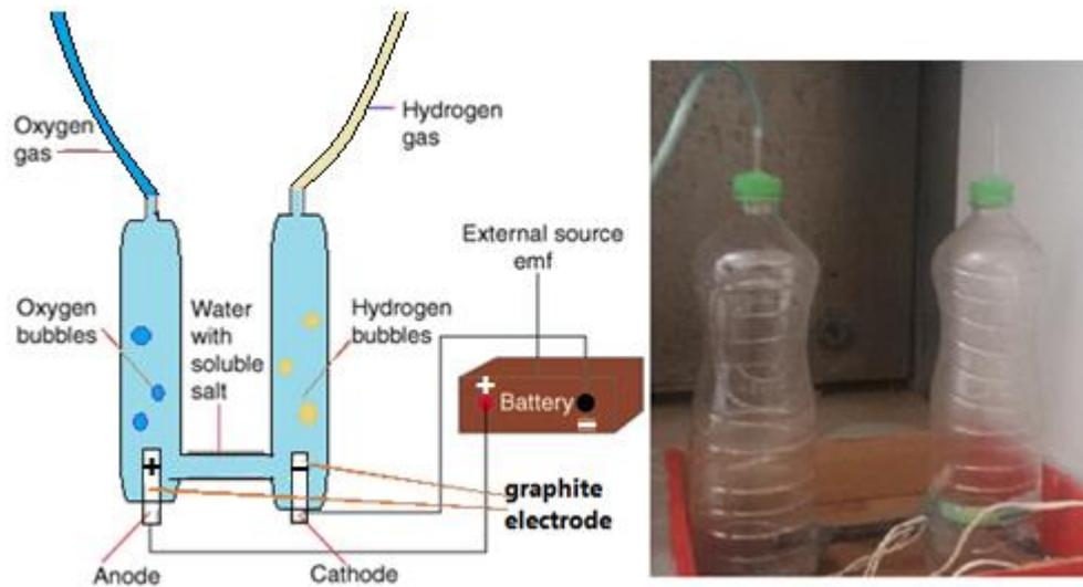
Figure 3.7: water electrolysis: Hydrogen gas gathers at the cathode and Oxygen gas gathers at the anode. This is the plastic design.
