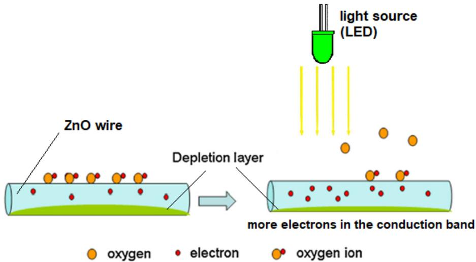
Figure 2.1: effect of light illumination on ZnO wire
